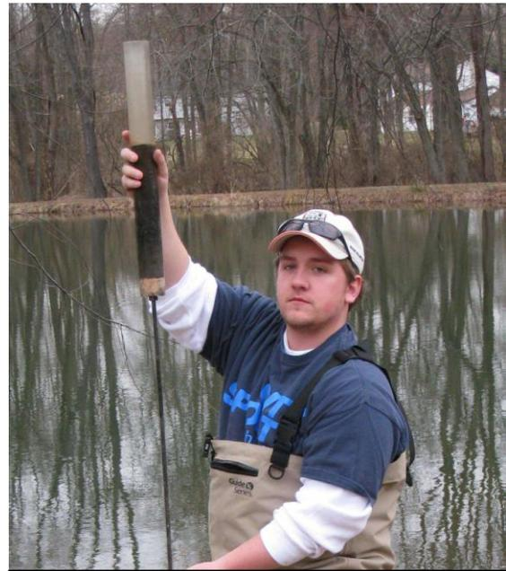
*Fig. 2 Andrew Brainard, with core tube and plunger used to extract pond sediments.*
