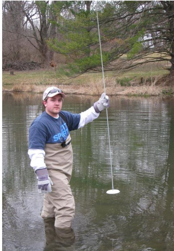
***Fig. 5. Metal probe used to determine current, and original, water depth at regularly spaced locations within each pond.***
