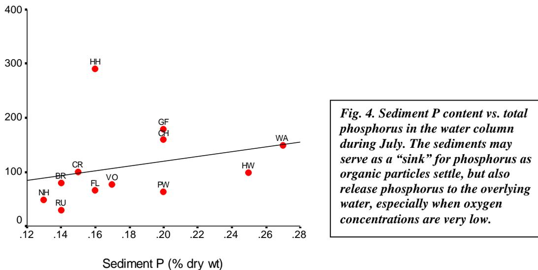
*Fig. 4. Sediment P content vs. total phosphorus in the water column during July. The sediments may serve as a “sink” for phosphorus as organic particles settle, but also release phosphorus to the overlying water, especially when oxygen concentrations are very low.*
