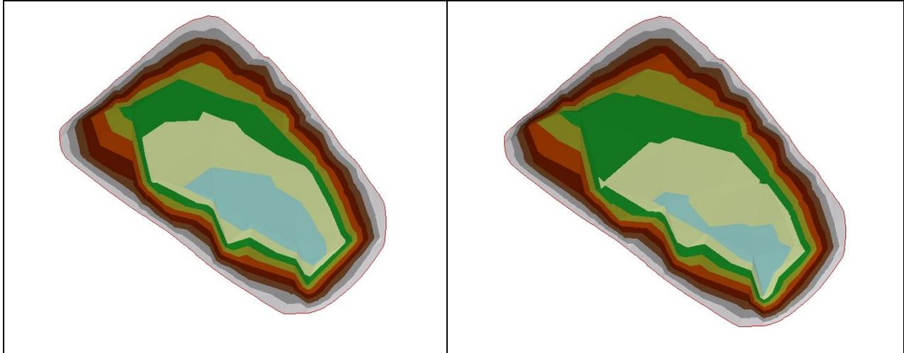
*Fig. 6. Original (L) and current (R) depth contours of one of the 10 ponds sampled for sediment characteristics and accumulation rates.*
